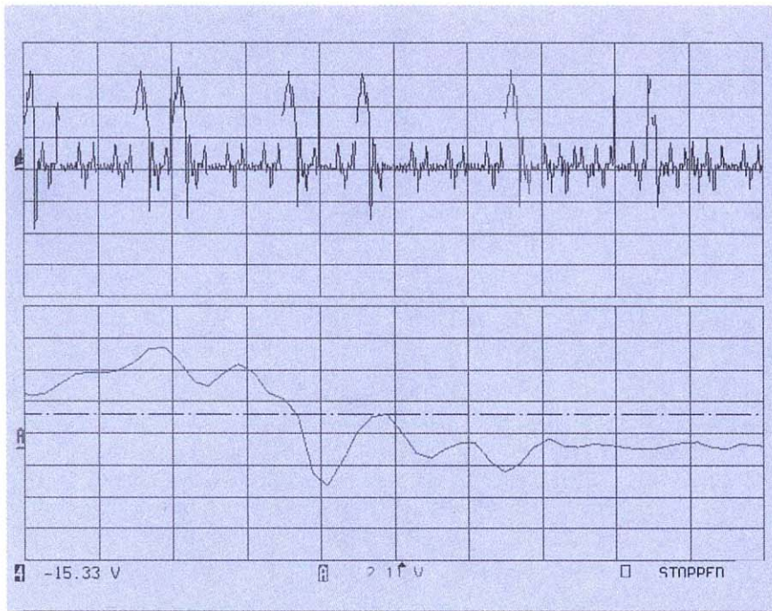
Figure 9. Sequence mode is used to examine a series of possible glitches. The Zoom trace A shows the details of a "bump" following a valid high-to-low transition.
